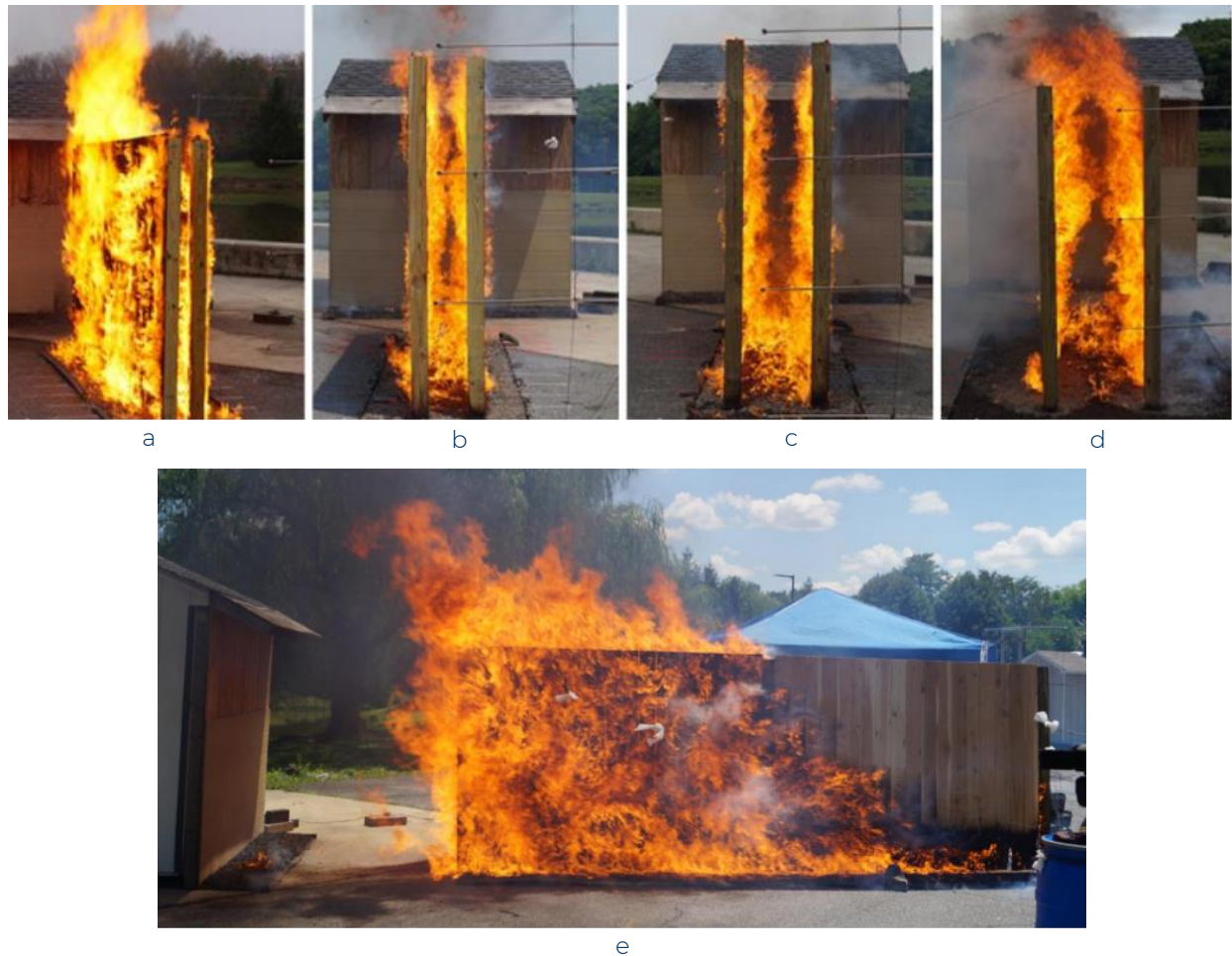
Figure 11. Fire behavior between parallel fences (a) 0.6 ft apart, (b) 1 ft apart, (c) 1.5 ft apart, (d) 2 ft apart, and (e) 3 ft apart and longer fence ( Butler et al., 2022 ), used with permission.
