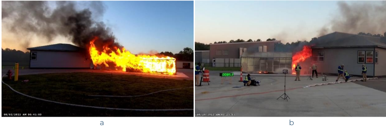
Figure 9. Photographs of a wind-driven building-to-building fire spread experiment at the IBHS Research Center showing (a) a burning woodshed positioned 30 ft from the main building and (b) a burning metal shed positioned 10 ft from the main building. In both cases, the open shed door is facing the main building.
